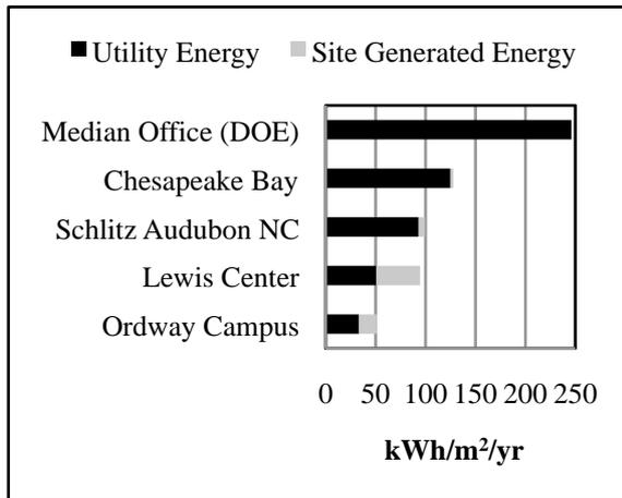
Figure 1 Energy Utilization of High Performance Buildings
