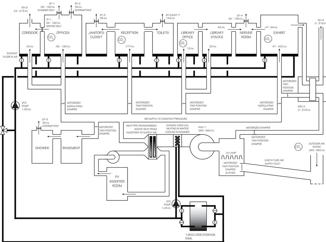
Figure 4 HVAC System Schematic, Load Side
