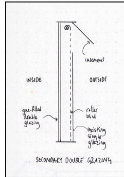
Figure 2 Secondary Double Glazing
