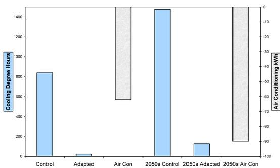
Figure 7 House Living Room: July CDH. The right hand axis shows air conditioning power consumption (in kWh) required to control overheating in the air conditioned cases.
