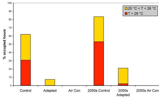
Figure 6 House Living Room: Percentage of July occupied hours exceeding CIBSE comfort temperature, 25 °C is shown by total size of bars. Hours during which the CIBSE overheating temperature, 28 °C, is exceeded are shown in red.
