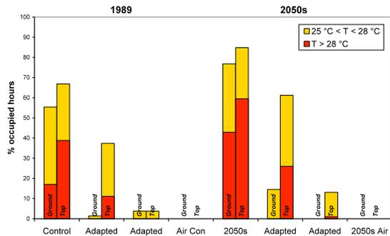
Figure 8 Living rooms in flats: Percentage of occupied hours exceeding CIBSE comfort temperature, 25 °C is shown by total size of bars. Hours during which the CIBSE overheating temperature, 28 °C, is exceeded, are shown in red.
