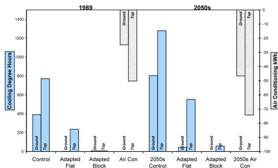
Figure 9 Flat Living Room: July CDH. The right hand axis shows air conditioning power consumption (in kWh) required to control overheating in the air-conditioned cases.
