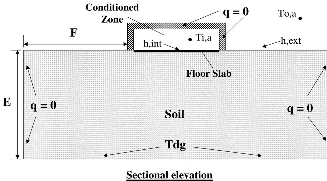
Figure 1 Geometry of a typical test problem (Neymark et al., 2008).
