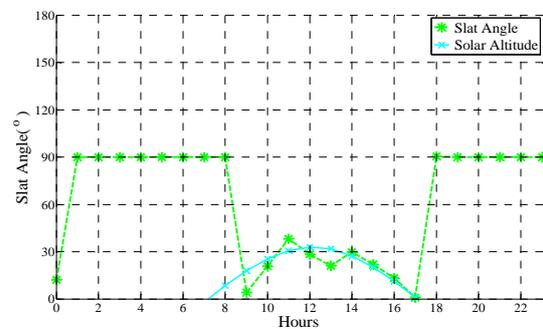
Figure 12 I-W-NDC Simulation result (slat angle)
