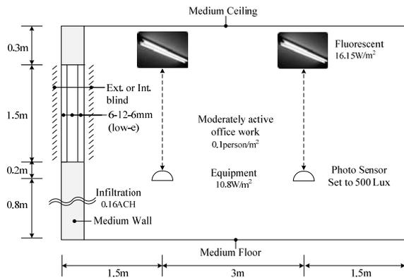
Figure 2 Simulation model
