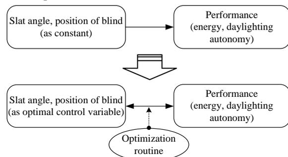
Figure 1 Optimal control of blind systems: From Steps 1, 2 to Step 3
