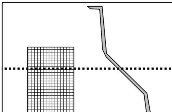
Figure 7. Wall with blocked up door and non-emerging crack. Analysis line is materialised by dotted line.
