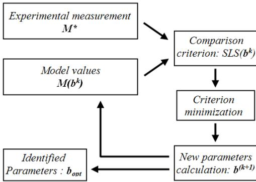
Figure 3. Estimation by inverse method principle.
