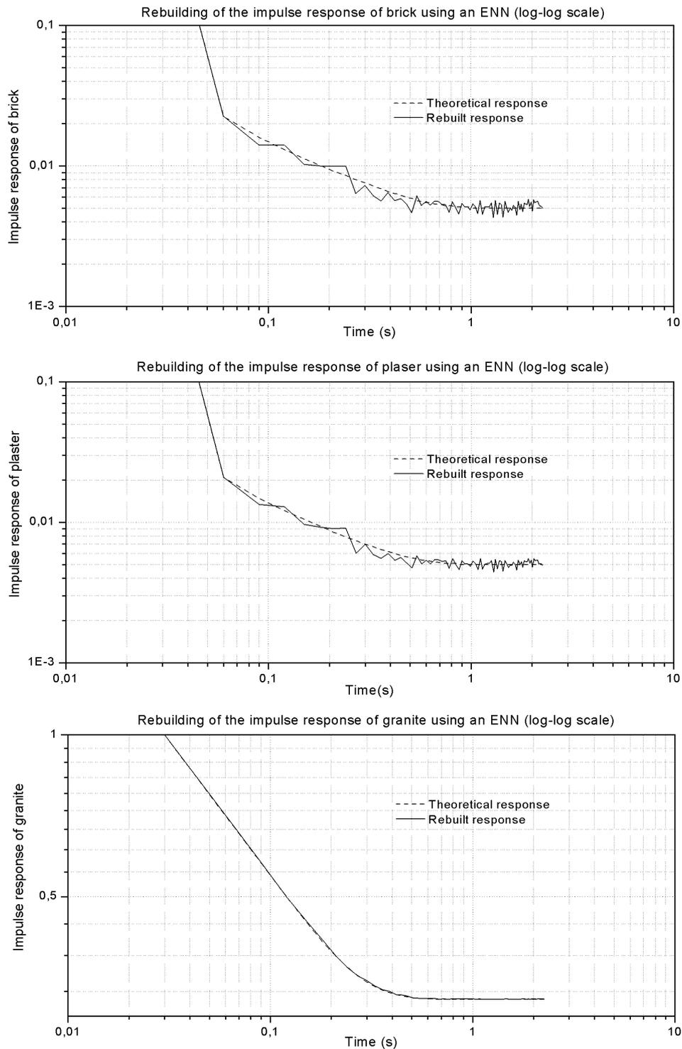
Figure 6. Rebuilt impulse responses of brick, plaster and granite (log-log scale).
