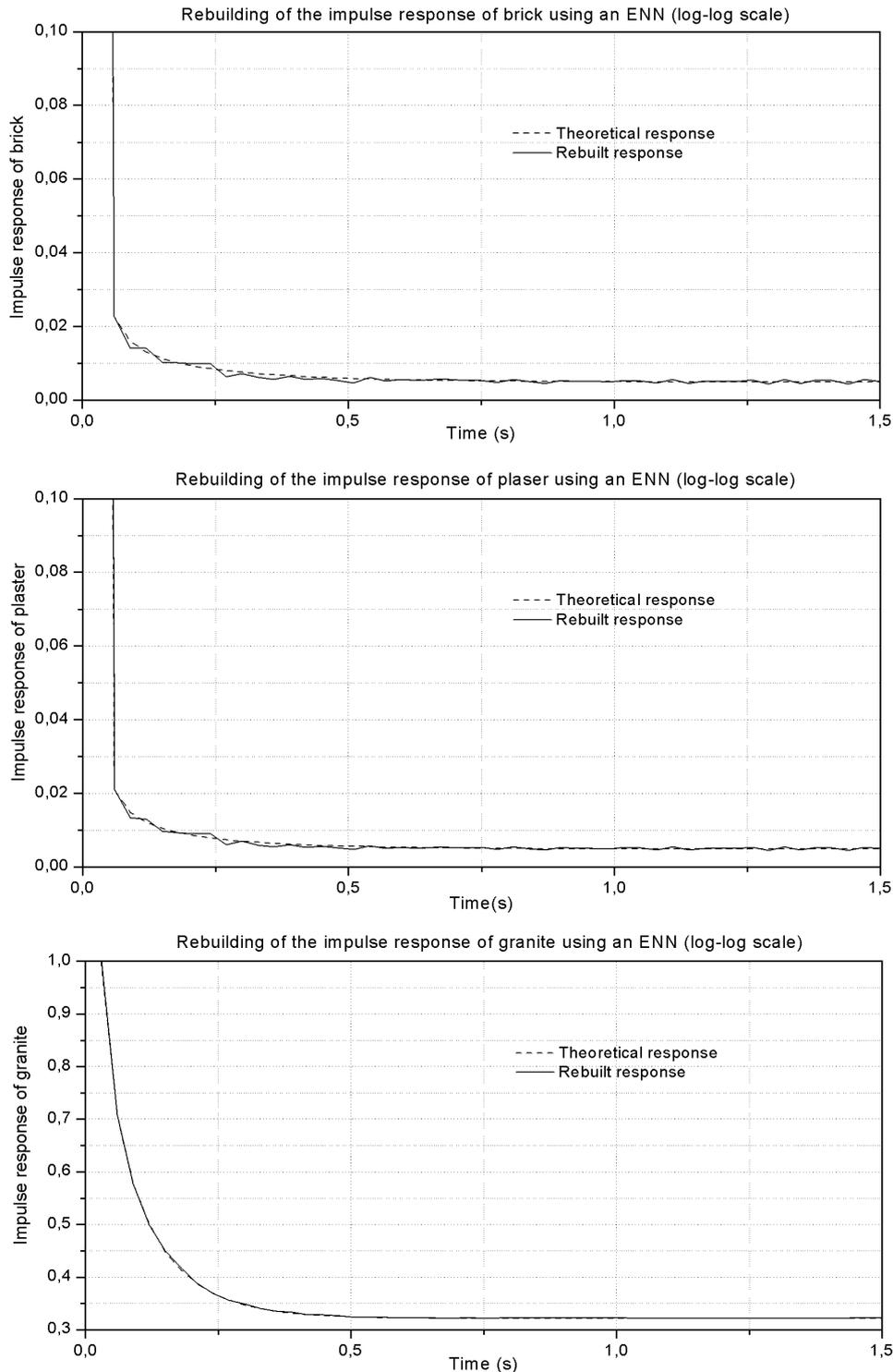
Figure 5. Rebuilt impulse responses of brick, plaster and granite (linear scale).
