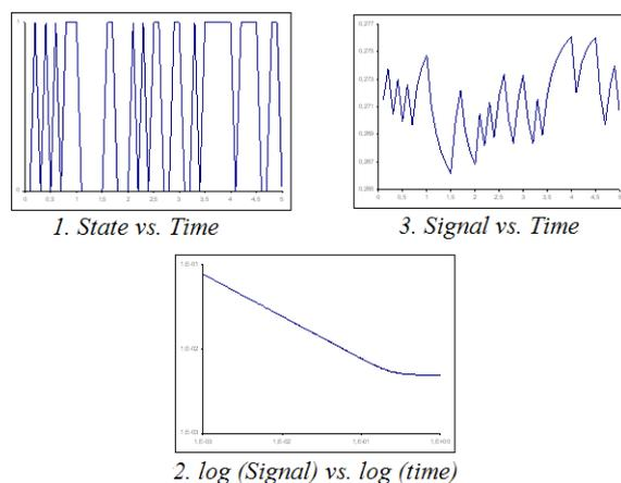
Figure 2. Examples: 1. PRBS, 2. Sample response to a pulsed stress, 3. Sample response to PRBS.
