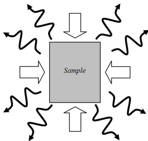
Figure 1. The photothermal experiment. White arrows: light excitation, black arrows: IR response.
