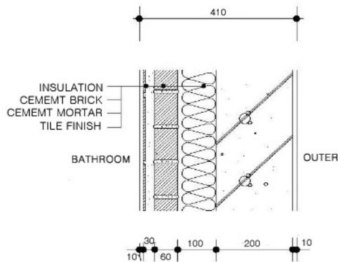
Figure 1 Typical structure of the outer wall
