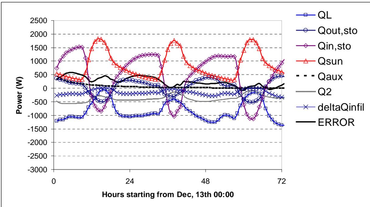
Figure 9 Audit model. Heat flows for the cool down period. In this figure,  $Q_L$  includes a base infiltration component,  $\text{delta}Q_{\text{infil}}$  is the variation of infiltration around the base component.  $Q_2$  is the sum of all the secondary heat flows not explicitly shown for clarity purposes.
