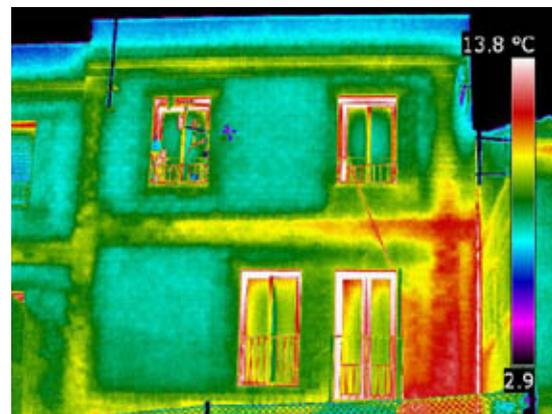
Figure 5 Infrared image of the south façade.
