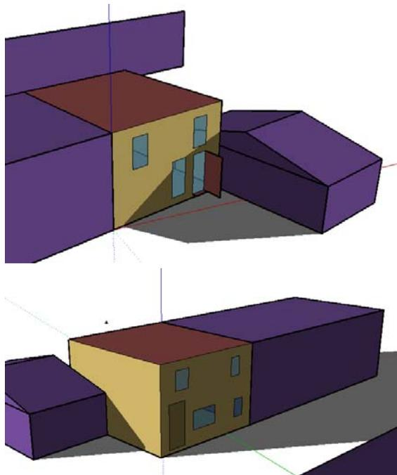
Figure 4 EnergyPlus model of the house, visualized with GoogleSketchUp. Upper image: view from south. Lower image: view from north.
