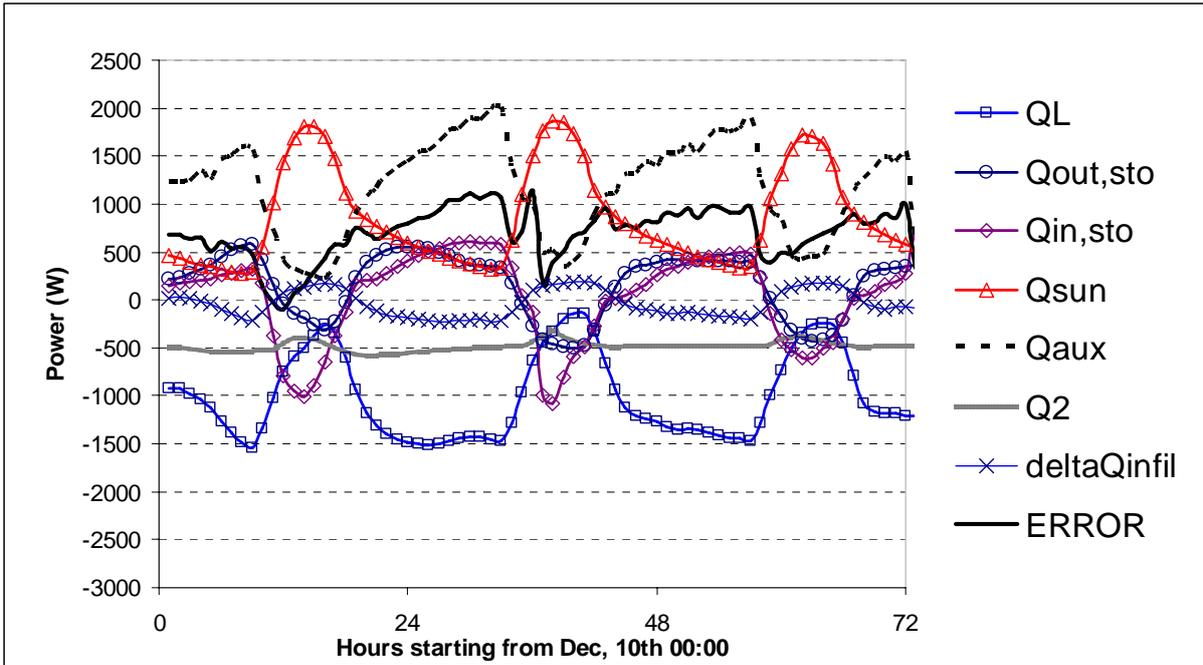
Figure 8 Audit model. Heat flows for the co-heating period. In this figure,  $Q_L$  includes a base infiltration component,  $\text{delta}Q_{\text{infil}}$  is the variation of infiltration around the base component.  $Q_2$  is the sum of all the secondary heat flows not explicitly shown for clarity purposes.
