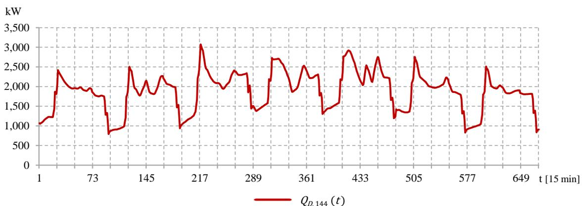
Figure 7: Total test district heating load profile
