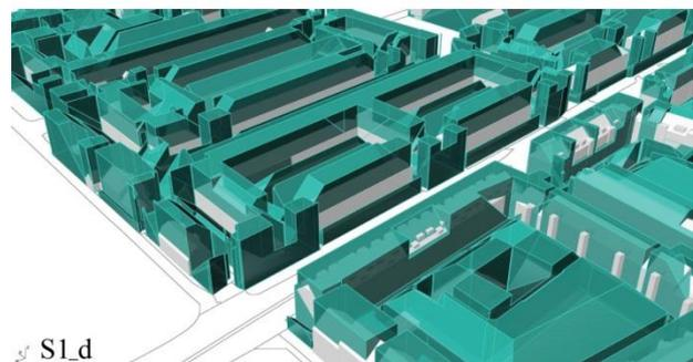
Figure 7: The illustrative sequence for the generation of theoretical maximum buildable potential: S1\_a) The application of building height constraint, S1\_b) The application of building distance, S1\_c) The application of visual access to the outside, S1\_d) The application of daylight access.
