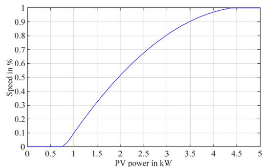
Figure 8: Polynomial for adapting the speed of MHPs
