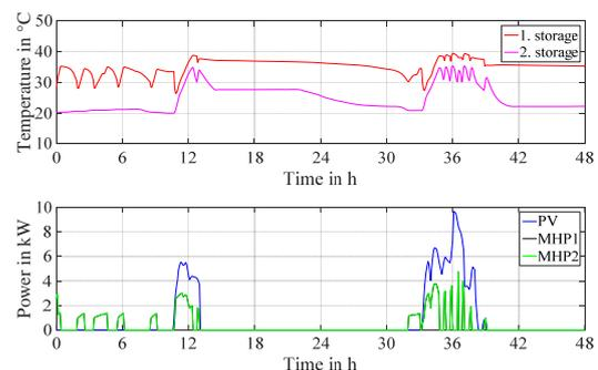
Figure 9: Adaption of MHPs to PV power during a period of 48 hours
