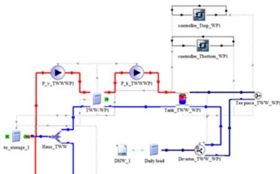
Figure 6: Detail of one domestic hot water heat pump and thermal storage system in the TRNSYS model
