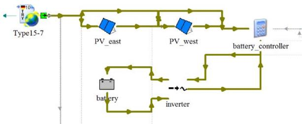
Figure 7: Detail of electrical production and storage system in the TRNSYS model
