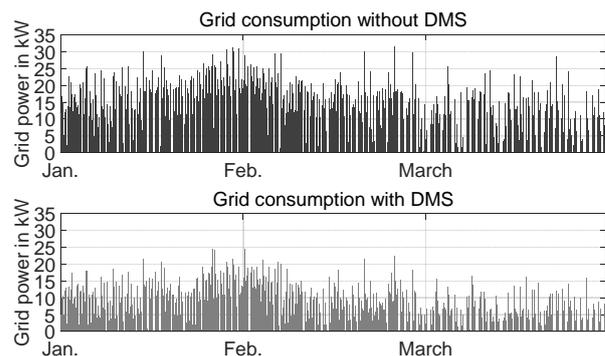
Figure 12: Grid consumption from January until March with and without DMS
