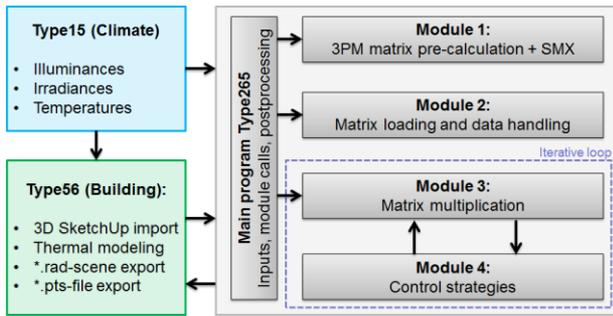
Figure 2: Artlight 2.0: model structure
