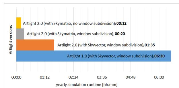
Figure 5: Runtime efficiency of Artlight implementation
