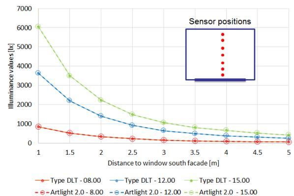
Figure 7: Validation results: Artlight 2.0 vs. Type DLT
