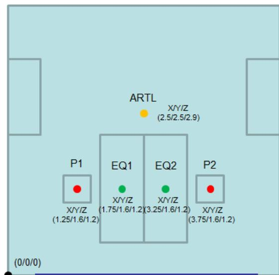
Figure 10: Geopositions of internal gains
