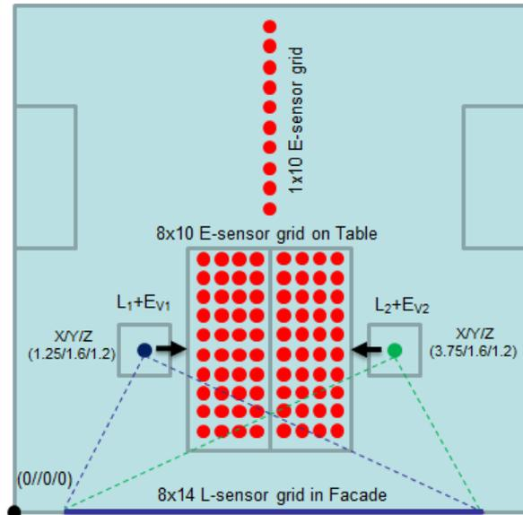
Figure 12: Sensor positions within the Radiance-scene
