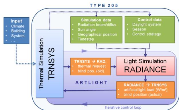
Figure 1: Scheme of simulation routine Artlight 1.0
