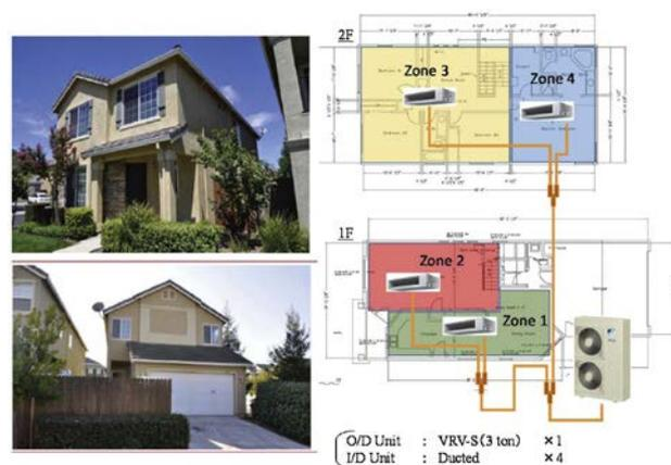
Figure 3 The facades and schematic layout of the Caleb House
