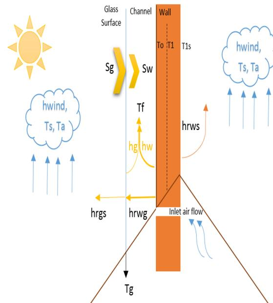
Figure 1: Physical model scheme of solar chimney.
