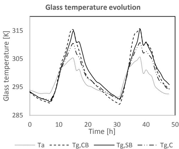
Fig. 7. Results of evolution of the glass temperatures with different materials.
