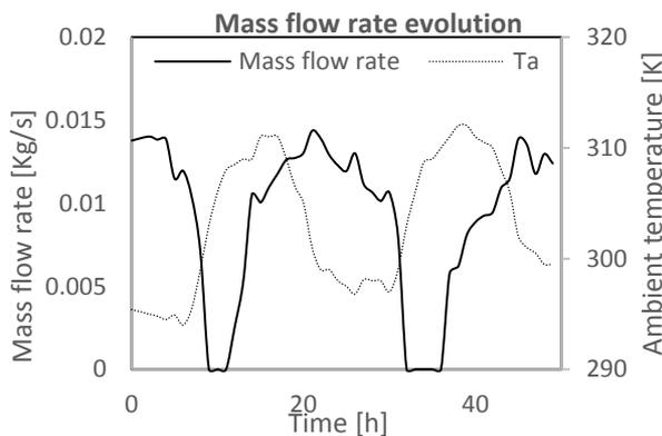
Figure 5: Mass flow that crosses the chimney.
