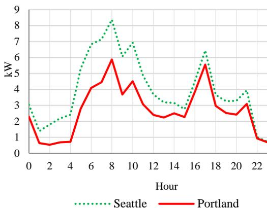
Figure 6: Comparison of 1,344 ft<sup>2</sup> Homes in Seattle and Portland with no PV or Battery Storage; January 8
