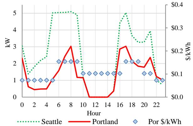
Figure 7: Comparison of 1,344 ft<sup>2</sup> Homes in Seattle and Portland with 15 kW of PV and 12 kWh of Battery Storage; January 8
