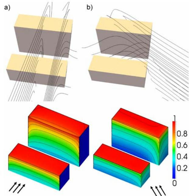
Figure 5: WDR deposition for two buildings with perpendicular and 45° oblique wind directions, a) and b) trajectories of 0.3 mm droplets and c) catch ratio for rain intensity of 1 mm/h at 3 m/s wind speed.
