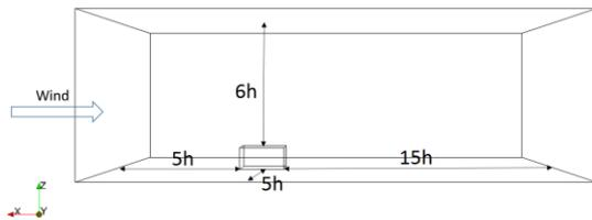
Figure 1: Computational domain setup.
