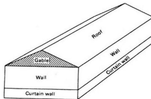
Figure 1: Typical A-frame greenhouse geometry
