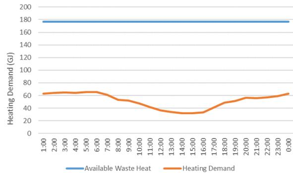
Figure 4: Comparison of hourly heating demand and available waste heat in a typical winter day (Jan. 3<sup>rd</sup>.)
