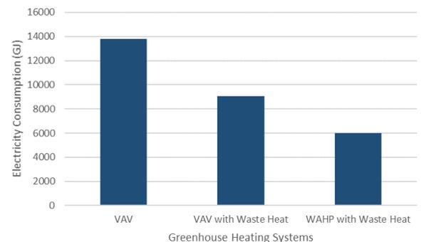
Figure 5: Annual Electricity used for Heating
