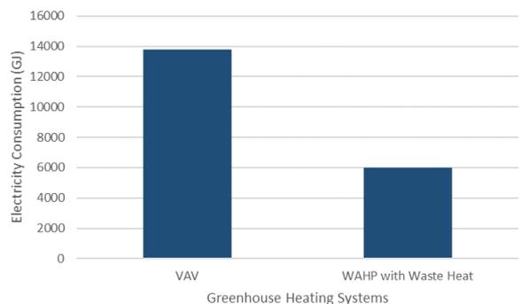
Figure 9: Annual Electricity Consumption for heating of electric VAV vs. WAHP, Waste Heat System
