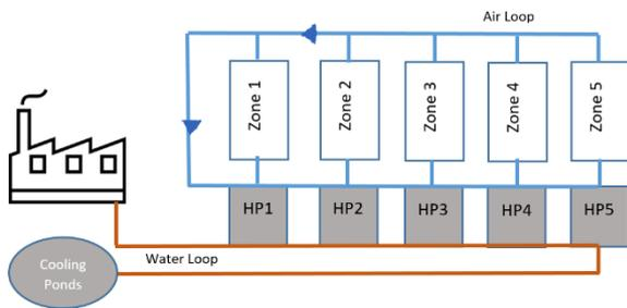
Figure 3: Schematic system diagram for water to air heat pump using waste heat
