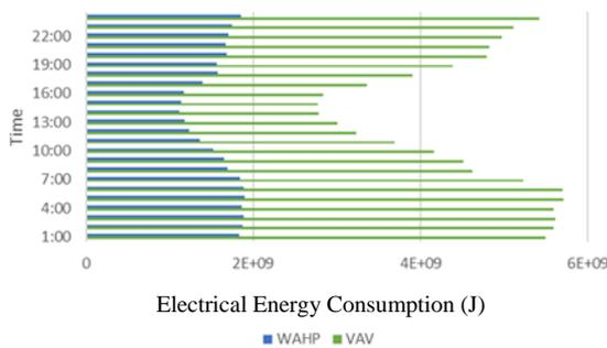
Figure 7: WAHP vs. VAV Hourly Electrical Consumption for Jan. 3<sup>rd</sup>.
