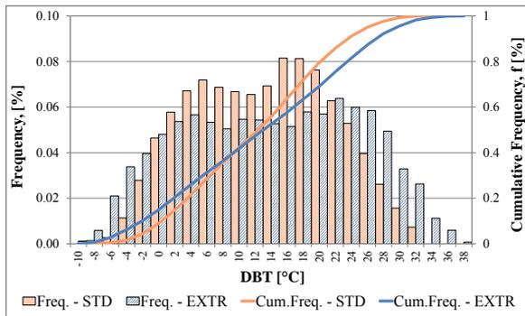
Fig. 2 – External Dry Bulb Temperature – Bolzano.
