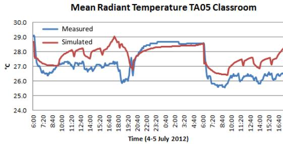
Fig. 8 – Comparison between predicted and measured mean radiant temperature
