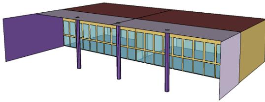
Fig. 4 – Sketch of simulated thermal zones
