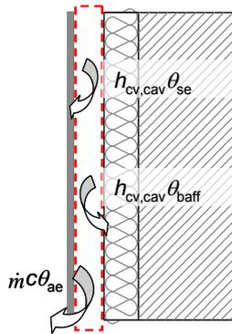
Fig. 4 – Cavity air heat balance scheme
