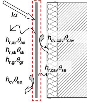
Fig. 3 – Baffle surface heat balance scheme
