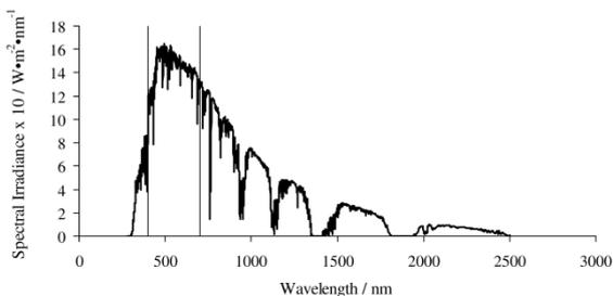
Fig. 1 – Terrestrial global spectrum, AM 1.5,  $1000 \text{ W}\cdot\text{m}^{-2}$  – based on ASTM G173-03 (ASTM, 2008)
