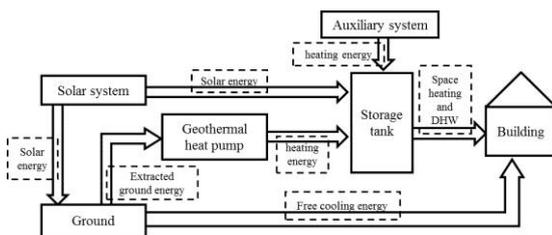
Fig. 3 – SAGSHP simplified scheme. Generic diagram
