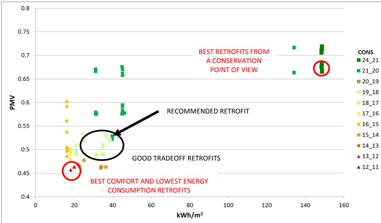
Fig. 6 – Optimal retrofit solutions up to the 20<sup>th</sup> generation
