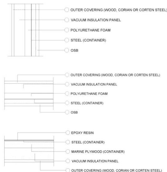
Fig. 3 – Coverage, wall and floor stratigraphies.
