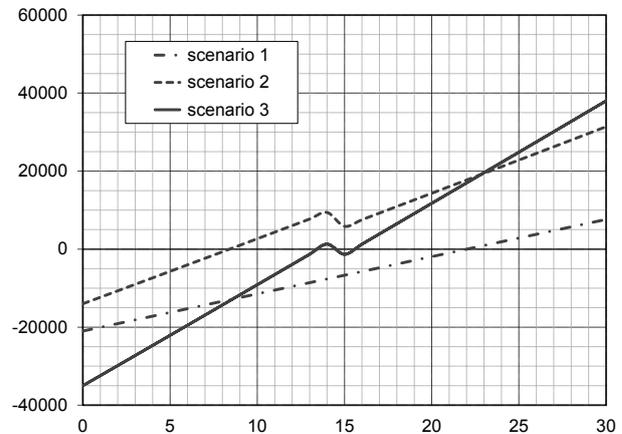
The deflection of the curves of Scenario 2 and 3 at the end of year 14 is due the cost of the replacement of the heat recovery and extraordinary maintenance at year 15.
