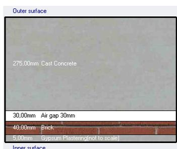
Fig. 4 – Drawing of the external wall construction
