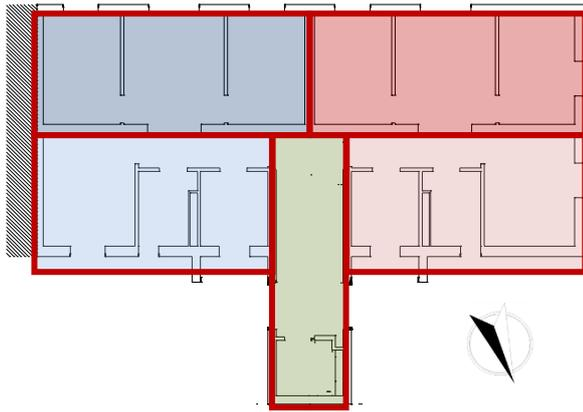
Fig. 6 – Thermal zoning of a typical floor
