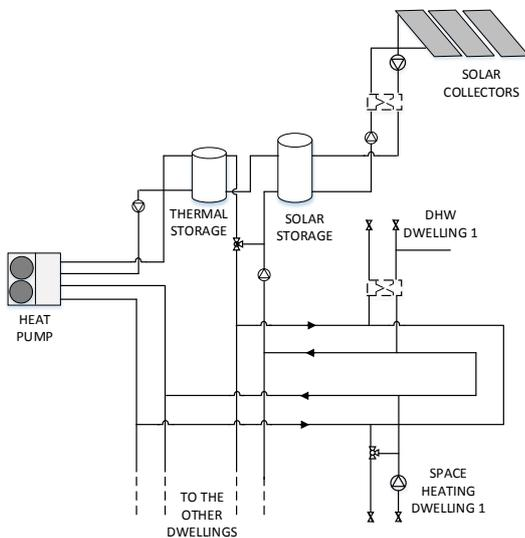
Fig. 7 – Sketch of the TRNSYS deck: building + generation and distribution system + control system
