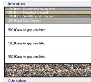
Fig. 5 – Drawing of the ground floor construction
