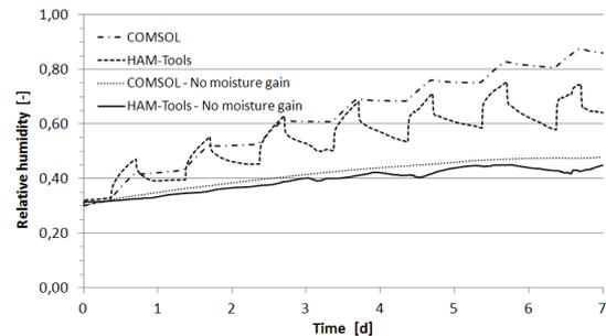
Figure 4 – Relative humidity trend for a 0.5 h<sup>-1</sup> ventilation rate. COMSOL and HAM-Tool results for scenarios with and without moisture gain
