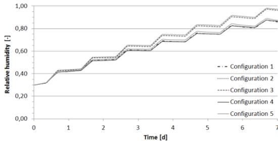
Figure 7 – Relative humidity trend for a  $0.5 \text{ h}^{-1}$  ventilation rate. COMSOL results for scenarios with different vents configurations
