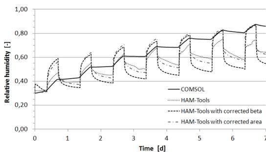
Figure 5 - HAM-Tools calibration on the results previously obtained for the scenario with moisture gain. The graph shows both cases: 1) application of a correction factor  $C_\beta = 0.4$  to the indoor surface moisture transfer coefficient  $\beta_{int}$ ; 2) and reduction of the building components area (-40 %)
