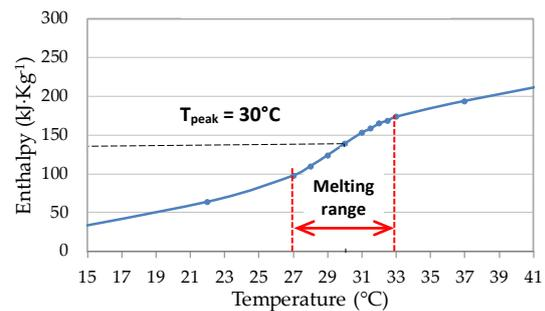
Fig. 1 – Enthalpy per unit mass for the PCM wallboards
