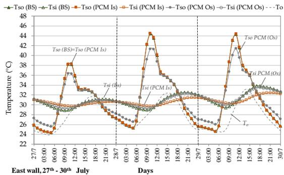
Fig. 6 – Inner and outer surface temperature of east wall (PCMs)
