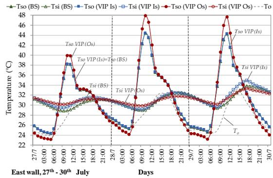
Fig. 5 – Inner and outer surface temperature of east wall (VIP)
