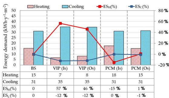
Fig. 4 – Energy needs for space heating and space cooling
