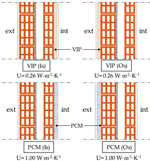
Fig. 3 – Wall configurations with VIPs and PCM on the inner surface (Is) and outer surface (Os)
