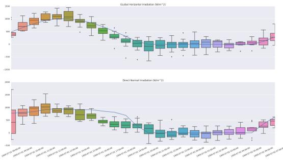
Fig. 3 – Forecast of 10 direct normal and global horizontal irradiance scenarios for 24 hours starting on July 1<sup>st</sup> in Golden, CO
