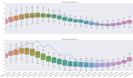
Fig. 4 – Forecast of 50 dry-bulb temperature predictions for Golden, CO (temperate, dry) and Atlanta, GA (hot, humid)
