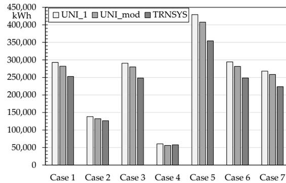
Fig. 4 – Rome: comparison among the cooling energy requirements (in kWh per year) for the reference building determined with ordinary  $a_C$  values (UNI\_1), the proposed  $a_C$  values (UNI\_mod) and with TRNSYS
