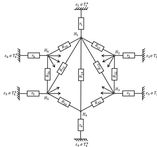
Fig. 3 – Model for long-wave radiation exchange with 6 surfaces
