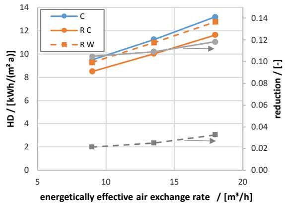
Fig. 7 – Heating demand (HD) for the small radiative heater on the ceiling (R C) and wall (R W) and reduction with respect to convective heating (C) depending on the energetically effective air exchange rate
