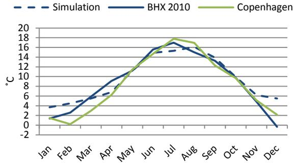
Figure 3: Comparative dry-bulb temperature for simulated and actual weather
