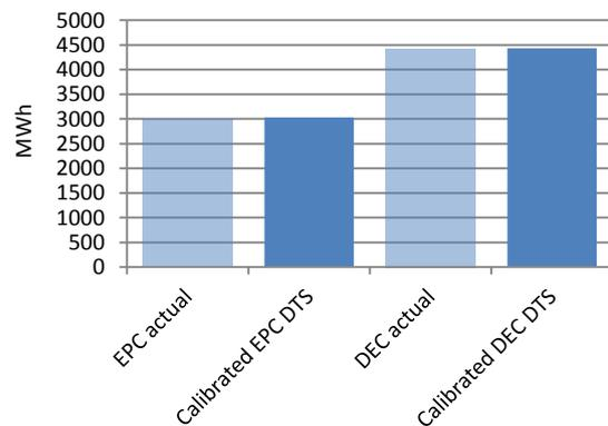
Figure 4: Final annual energy consumption from EPC, DEC and calibrated DTS models
