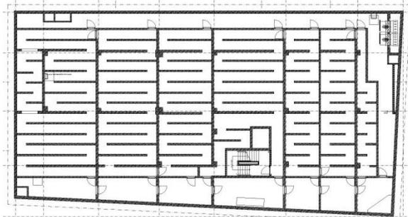
Figure 5 The labyrinth system layout located at the basement floor of the building
