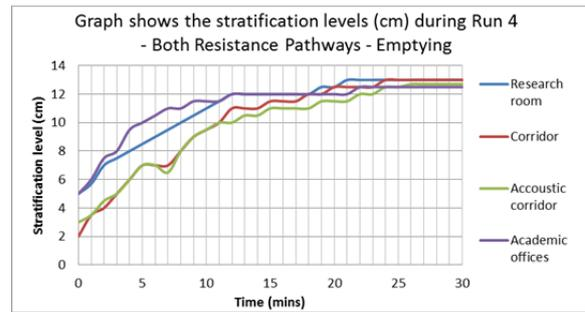
**Figure 7 - Graph shows the differences in stratification levels across the four zones of the scale model during the fourth run of the salt-bath model experiments.**
