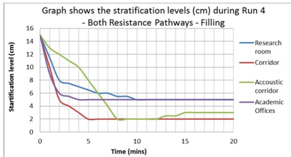
**Figure 6 - Graph shows the varying stratification levels in each of the four zones during the filling stage of the scale model.**
