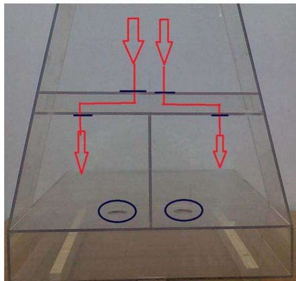
**Figure 2 - Image shows part of the scale model, highlighting the obstruction to air flow caused by the acoustic corridor of the academic offices. Red lines and arrows depict airflow; Blue lines highlight the model openings.**
