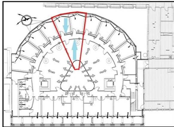
**Figure 1 - Image shows a plan view of the SSEES building (Short et al. 2009). The resistance pathways are indicated in this image by blue arrows, while the red boundary line depicts the section of the building to be modelled.**
