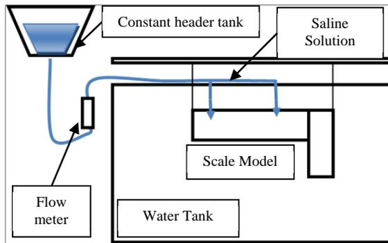
Figure 4 - Image shows experimental setup
