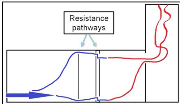
**Figure 3 - A schematic side view of the scale model, showing the airflow through the building while navigating through the resistance pathways.**
