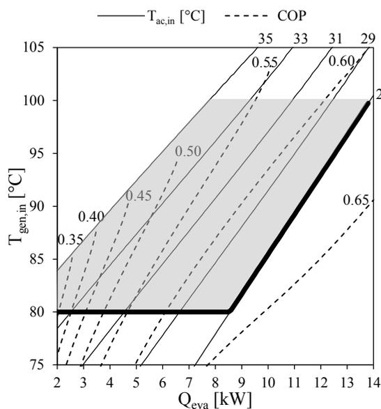
Figure 5 Chiller performance diagram (for  $T_{eva,out}=7^{\circ}\text{C}$ )
