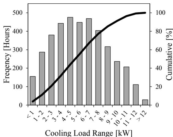
Figure 4 Cooling load distribution diagram
