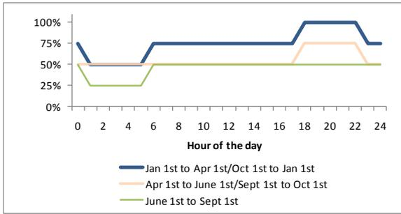
Figure 4 Load profile; lighting and plug loads.
