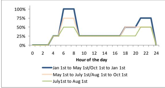
Figure 3 Load profile; hot water.
