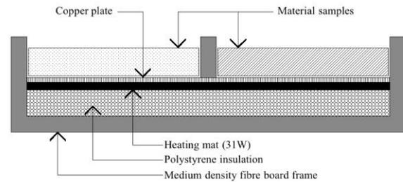
*Figure 1 Section through the test board*
