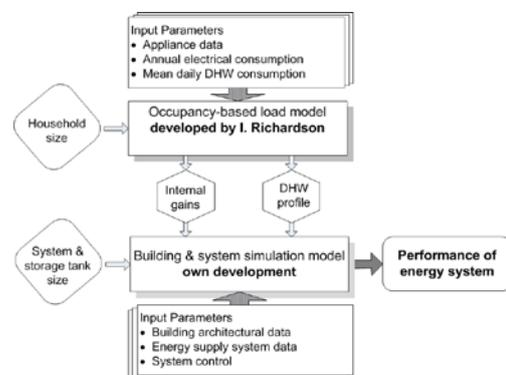
Figure 1: Methodological framework coupling occupant loads with building simulation
