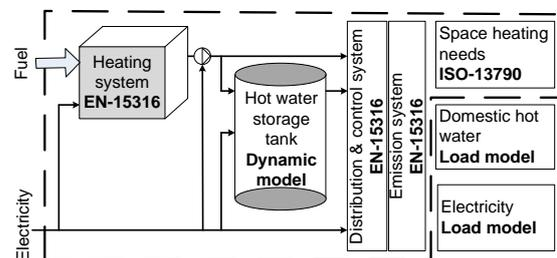
Figure 3: Generic energy flow diagram: Calculation started from left side where energy needs for space heating are computed and then different systems losses are taken into account. Profile for DHW draw-off and internal heat gains from non-HVAC electrical loads are generated using an external model.
