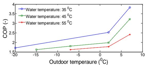
Figure 4: Coefficient of performance (COP) of the heat pump at standard test points (Mitsubishi Electric)
