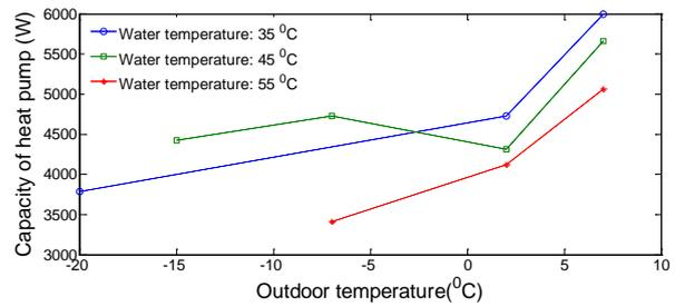
Figure 5: Heating capacity of the heat pump at standard test points (Mitsubishi Electric)
