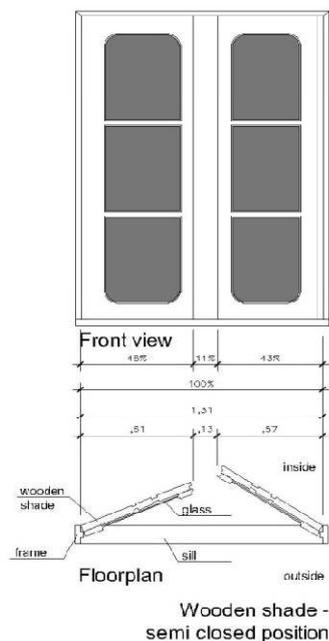
Figure 10 - window shade airflow permeability
