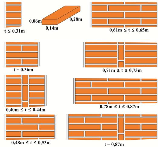
Figure 5 – Composition of the different thicknesses of the walls
