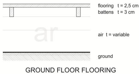
Figure 7 – flooring of the ground
