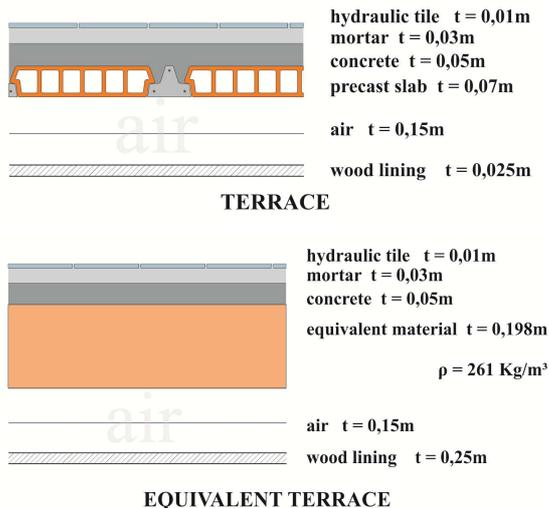
Figure 8 – Terrace and equivalent terrace
