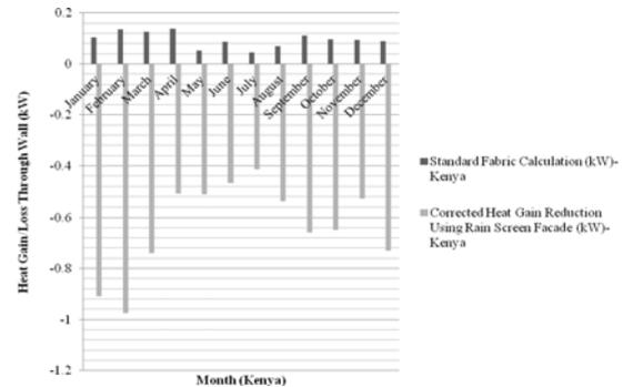
Figure 10- Wall Heat Gain Analysis comparing RSF against Standard wall in Kenya
