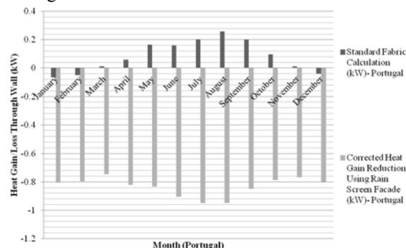
Figure 9- Wall Heat Gain Analysis comparing RSF against Standard wall in Portugal
