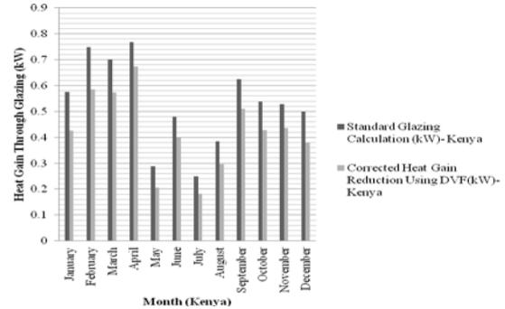
Figure 8- Heat Gain Analysis comparing DVF against Standard glazed external wall in Kenya
