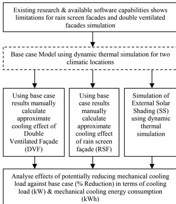
Figure 1- Mechanical Cooling Reduction Using Passive Systems Methodology Flow Diagram
