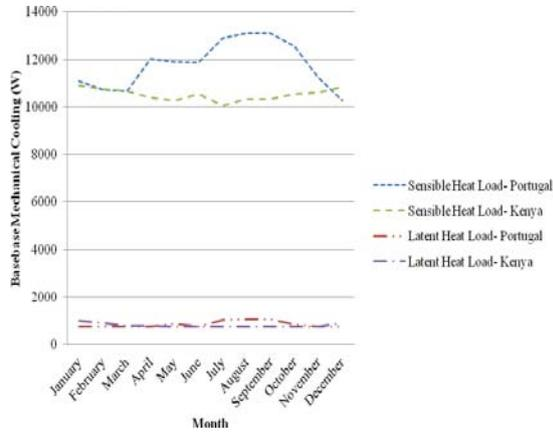
Figure 4- Base Case cooling loads for both climates
