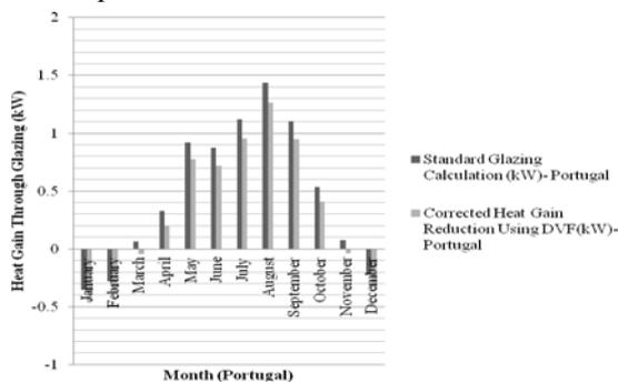
Figure 7- Heat Gain Analysis comparing DVF against Standard glazed external wall in Portugal
