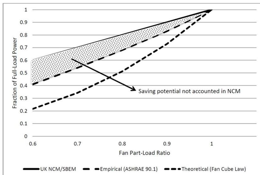
Figure 4 Demand-controlled ventilation saving potential not accounted in NCM
