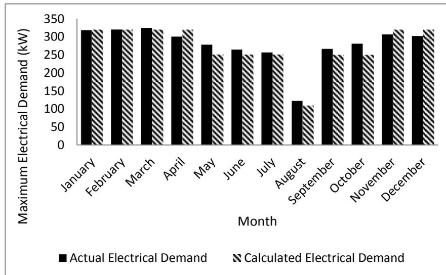
Figure 3 Maximum monthly electrical demand: Measured vs. Calculated
