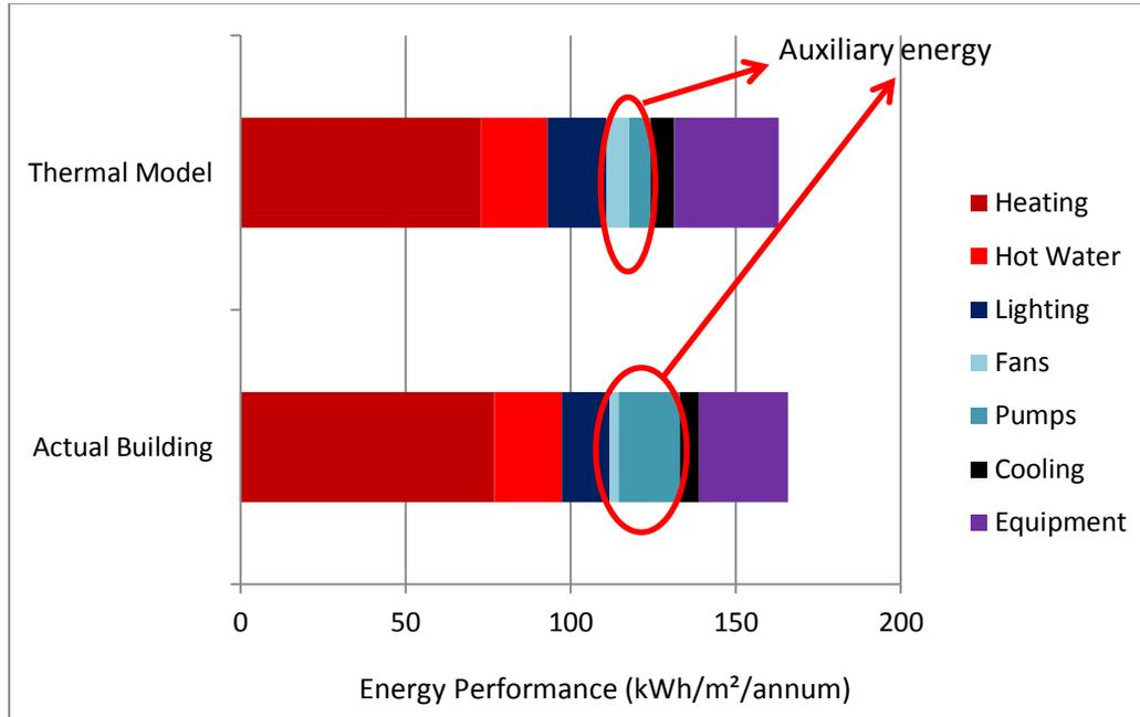
Figure 2 Actual vs. NCM-modelled energy performance of the case study building
