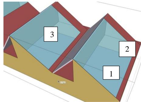
Figure 5 Area occupied by 35 Sanyo HIT-N240SE10 panels. The first roof surface (1&2) does not suffer from shading while the second area does (Apt 3, 44.13m<sup>2</sup>).
