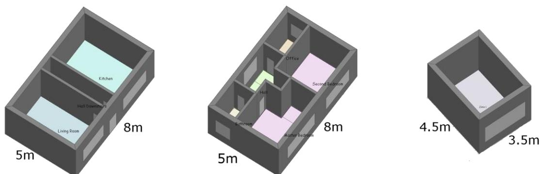
Figure 2 (left) Residential ground floor (middle) Residential 1<sup>st</sup> floor (Right) Office - Not To Scale
