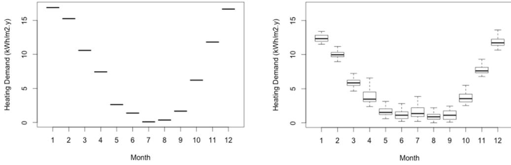
Figure 3 Office monthly heating demand box plots (left) Single deterministic (right) MAS Platform 50 replicates
