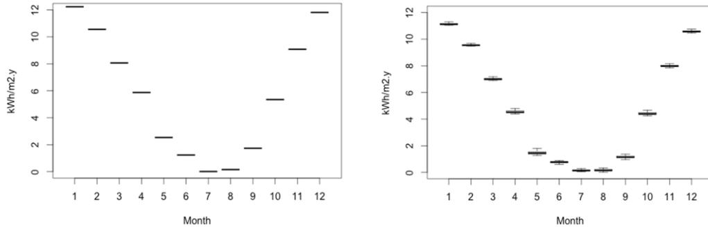
Figure 4 House monthly heating demand box plots (left) Single deterministic (right) MAS Platform 50 replicates
