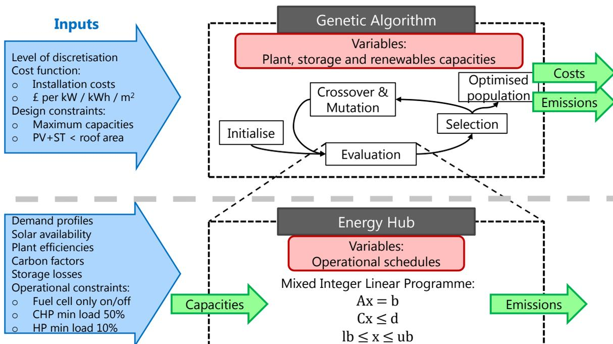
Figure 1. Schematic of the bi-level design and operational optimisation process.
