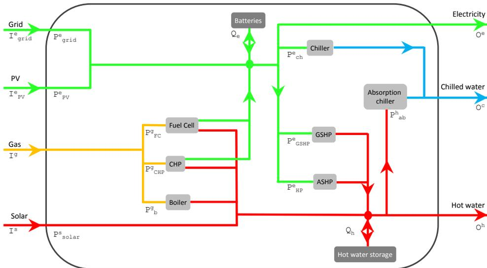
Figure 2. Schematic of the plant layout options considered in the energy centre. Inputs  $I$ , conversions  $P$ , storage  $Q$  and outputs  $O$  are indicated.
