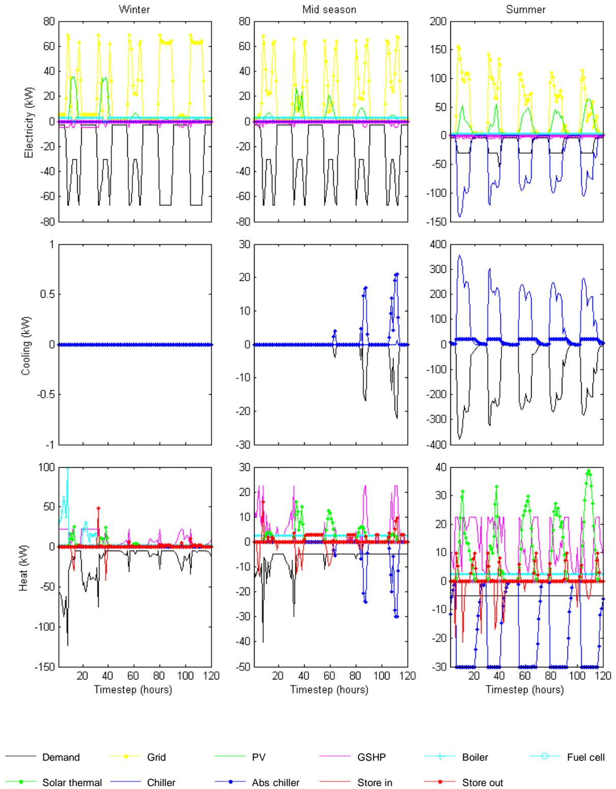
Figure 5. Results of the operational optimisation for an example design solution (highlighted in Figure 4). Energy balances are shown for electricity, cooling and heating for the winter, mid-season and summer periods.
