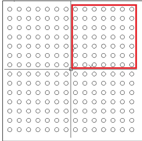
Figure 5 Energy piles layout, the size of the field was 58.5 x 58.5 m and the distance between piles 4.5 m.
