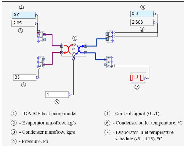
Figure 3 Parameter identification model
