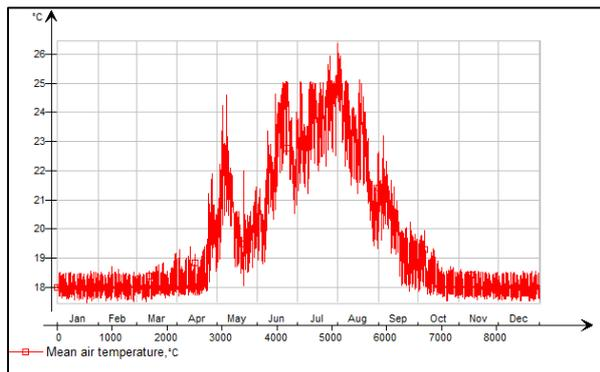
Figure 12 Indoor air temperature
