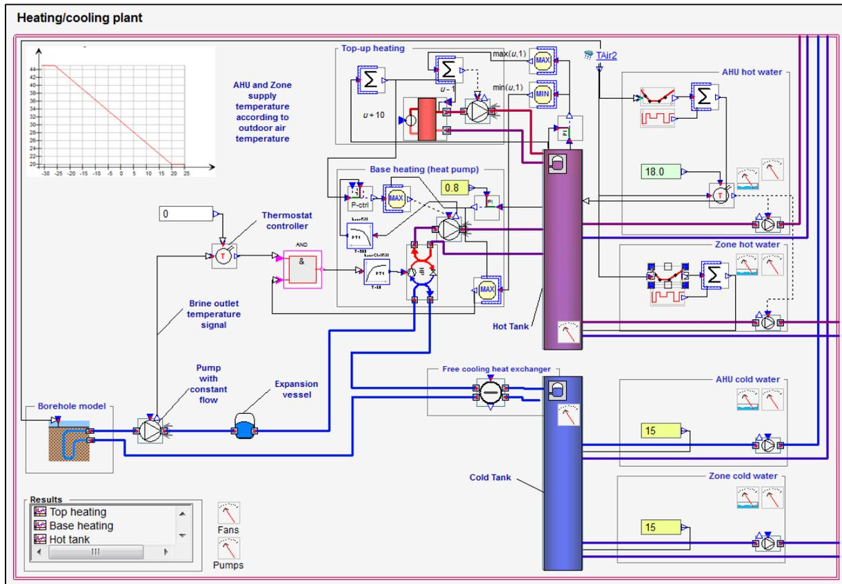
Figure 10 Detailed heating/cooling plant modelled in IDA
