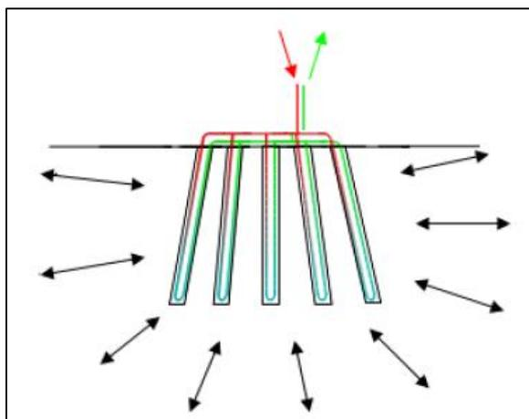
Figure 4 Heat flows in borehole model
