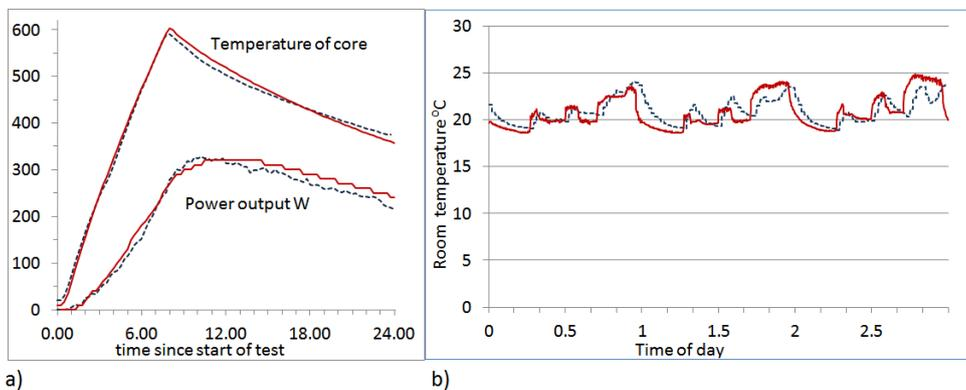
Figure 5: Calibration of heater models a) laboratory test data and b) field measurements. Solid lines show simulation, dotted lines measurements.
