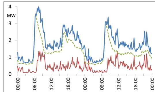
Figure 2: Heat demand profile (bold line) over 2 days for large estate, made up of space (dotted line) and water (narrow line) heaters.
