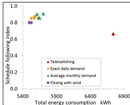
Figure 6: Total heat consumption and schedule following January to April under various fixed-timing charging approaches for the poorly insulated bungalow.
