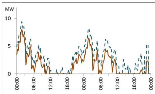
Figure 4: Ideal charging profiles for same 2 days optimised over 24 (solid) and 48 hours (dotted line).
