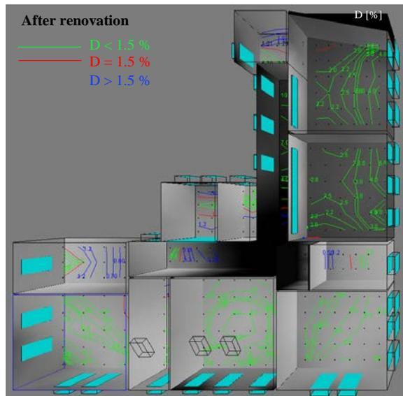
Figure 3 Daylight simulation outputs, D [%]
