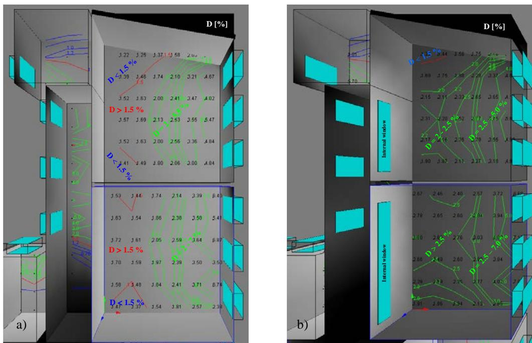
Figure 4 Daylight simulation in classrooms 1 and 2; a) before renovation and b) after renovation
