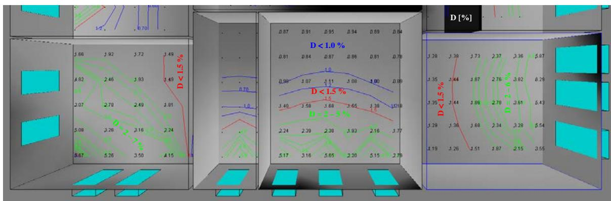
Figure 5 Daylighting in classrooms 3 to 5; before renovation
