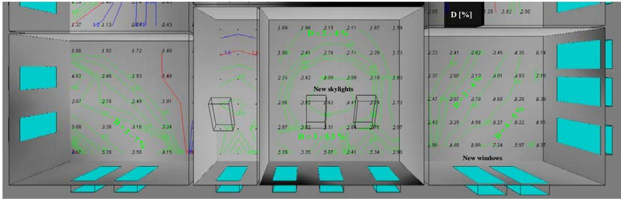
Figure 6 Daylighting in classrooms 3 to 5; after renovation
