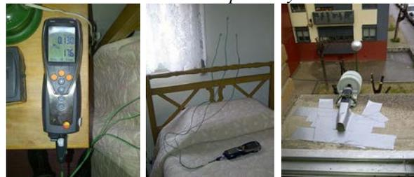
Fig. 4, 5 and 6. TESTO 435-2 instrument, instrument with three probes fixed on the inner surface of the façade and the wireless probe located in the external window sill respectively.
