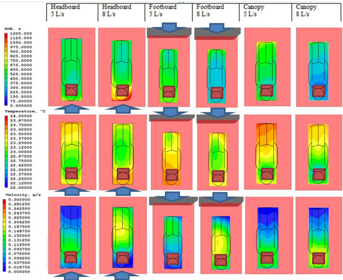
Figure 7 – A comparison of age of air, air velocity and temperature contours for different ventilation scenarios. Contours shown are from M1. Red box indicates breathing zone. Blue arrows represent supply airflow direction. Windows are positioned to the right of patients in the figure. Canopy system delivers air from above the BZ.
