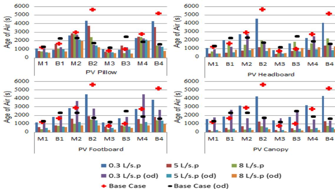
Figure 5 - Effect of PV system in comparison to the base case with and without the open door, as demonstrated by age of air (s).
