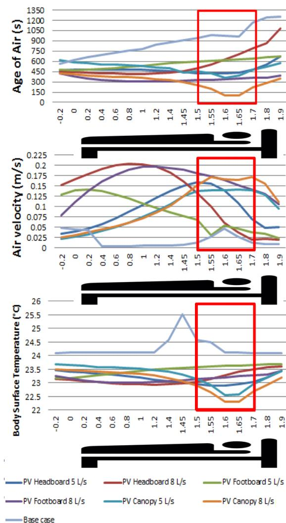
Figure 6 – Criteria assessment metrics at different distances from the patient's foot (metres) shown on x-axis. Red box indicates the BZ. Data are for M1.
