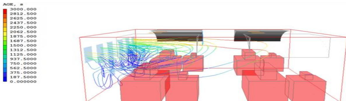
Figure 4 – Age of air streamlines realised from the windows in the base case scenario.
