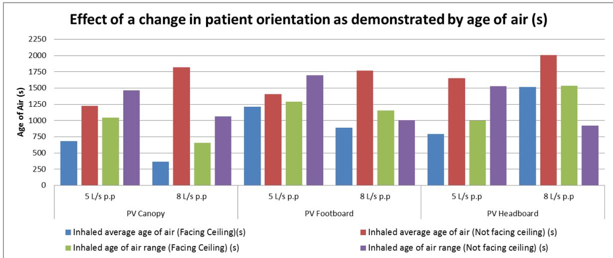
Figure 9 - Effect of a change in patient orientation on system performance, using age of air at the point of inhalation to indicate inhaled air quality.
