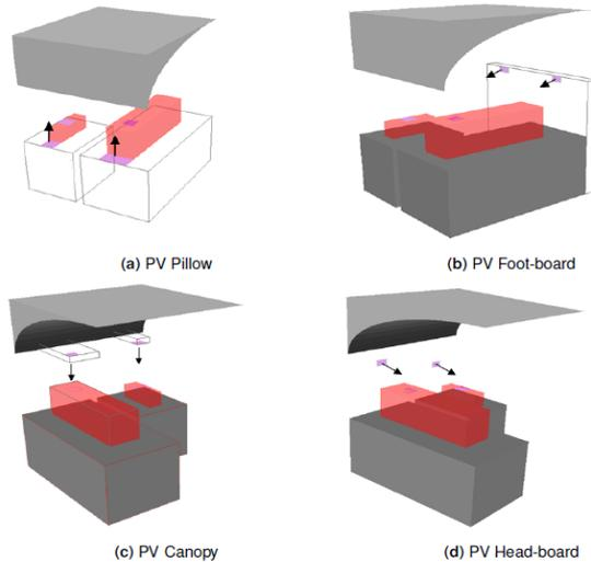
Figure 2 - PV Configurations. Arrows indicate the direction of the local mechanically supplied inlet air.
