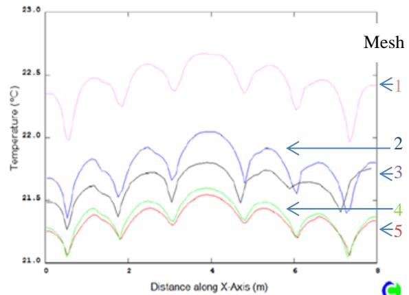
Figure 3 - Mesh Sensitivity Study. Average air temperature across the X-Axis at a height of 1.5m.
