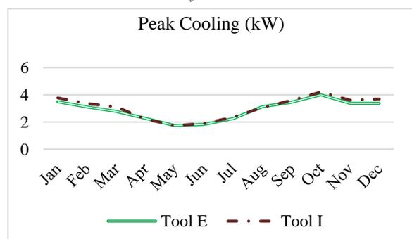
Figure 9: Peak cooling demand of equivalent models. Monthly breakdown
