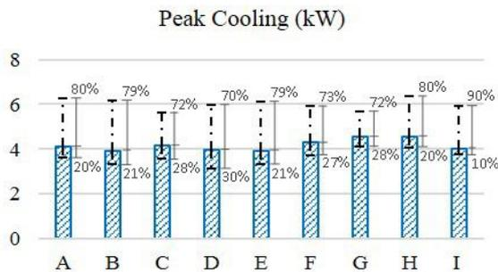
Figure 5: The graph demonstrates the results for peak hourly integrated cooling loads (kW). The bars illustrate the results for ICF, with the upper limit of the dashed line showing the peak cooling loads of the low mass construction and the lower limit showing the results of the high mass construction.
