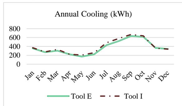
Figure 7: Annual cooling energy consumption of equivalent models. Monthly breakdown
