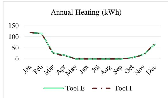
Figure 6: Annual heating energy consumption of equivalent models. Monthly breakdown
