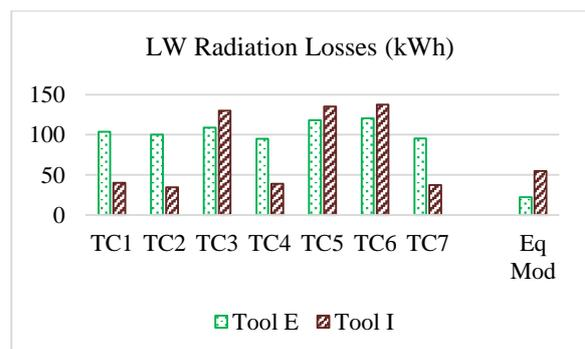
Figure 13: Long-wave radiation losses in South ICF wall
