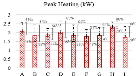
Figure 3: The graph demonstrates the results for peak hourly integrated heating loads (kW). The bars illustrate the results for ICF, with the upper limit of the dashed line showing the peak heating loads of the low mass construction and the lower limit showing the results of the high mass construction.
