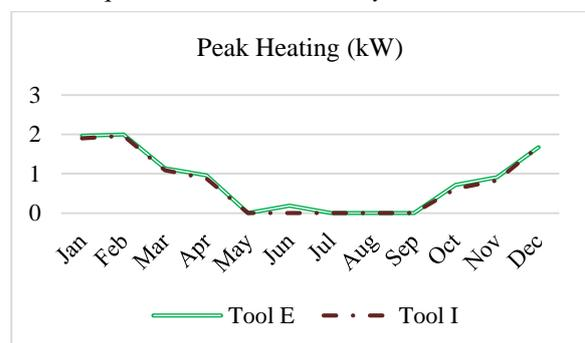
Figure 8: Peak heating demand of equivalent models. Monthly breakdown
