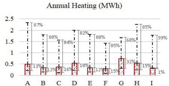
Figure 2: The graph demonstrates the results for annual heating energy consumption (MWh). The bars illustrate the results for ICF, with the upper limit of the dashed line showing the annual heating energy consumption of the low mass construction and the lower limit showing the results of the high mass construction.
