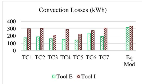
Figure 12: Convection losses in South ICF wall
